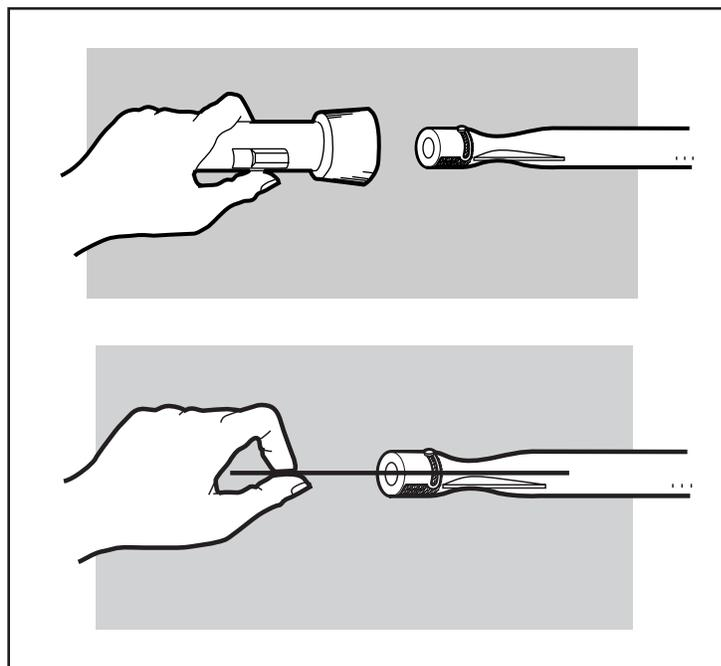
**REPLACING MAIN BURNERS**
