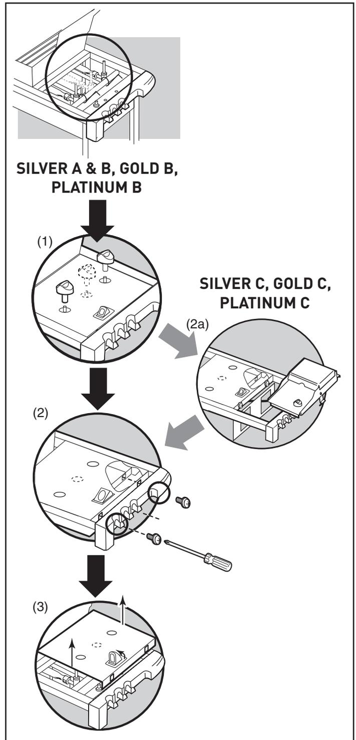
**CHECK THE FLEXIBLE HOSE TO MANIFOLD CONNECTION**
