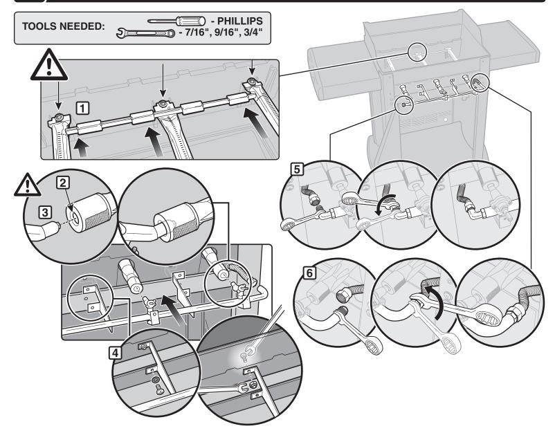
CAUTION: Burner tube openings (2) must be positioned properly over valve openings (3).
