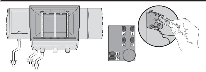
REASSEMBLY NOTE: After completely checking igniter wires, check for igniter spark. Push down on igniter button, listen for a clicking sound, and check for a spark at ceramic igniter. If you hear a click and see a spark, igniter module is working.
